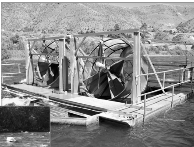
Above: Double rotary screw trap located just below the Old Monitor Bridge on the Wenatchee River.
