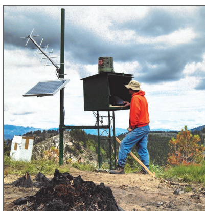
One of 10 newly installed rain gauges that alert residents of flash flood risk. Photo courtesy of USGS.
