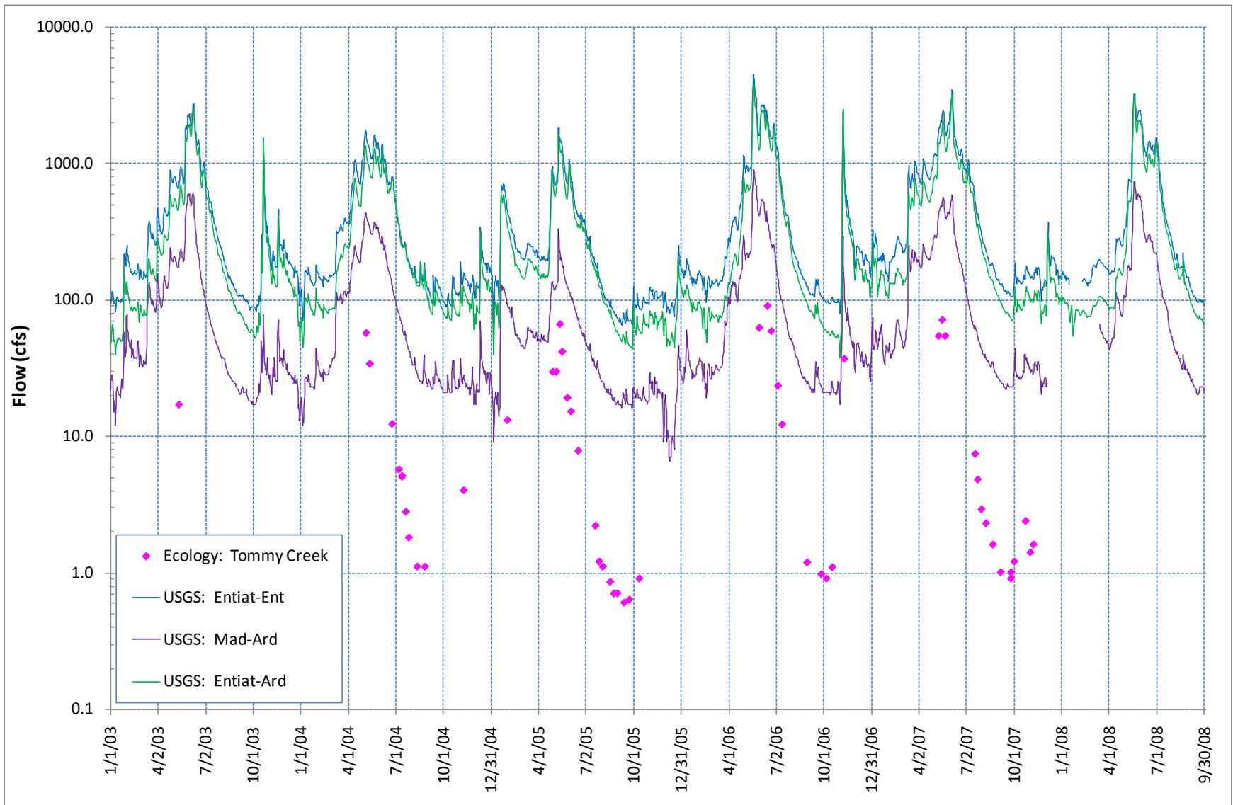
Figure 11. Measured flows at the “Tommy Creek below USFS Quarry” staff gage site, with USGS gaged flows.
